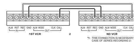
Figure 4. Connecting VCRs for Series Recording
